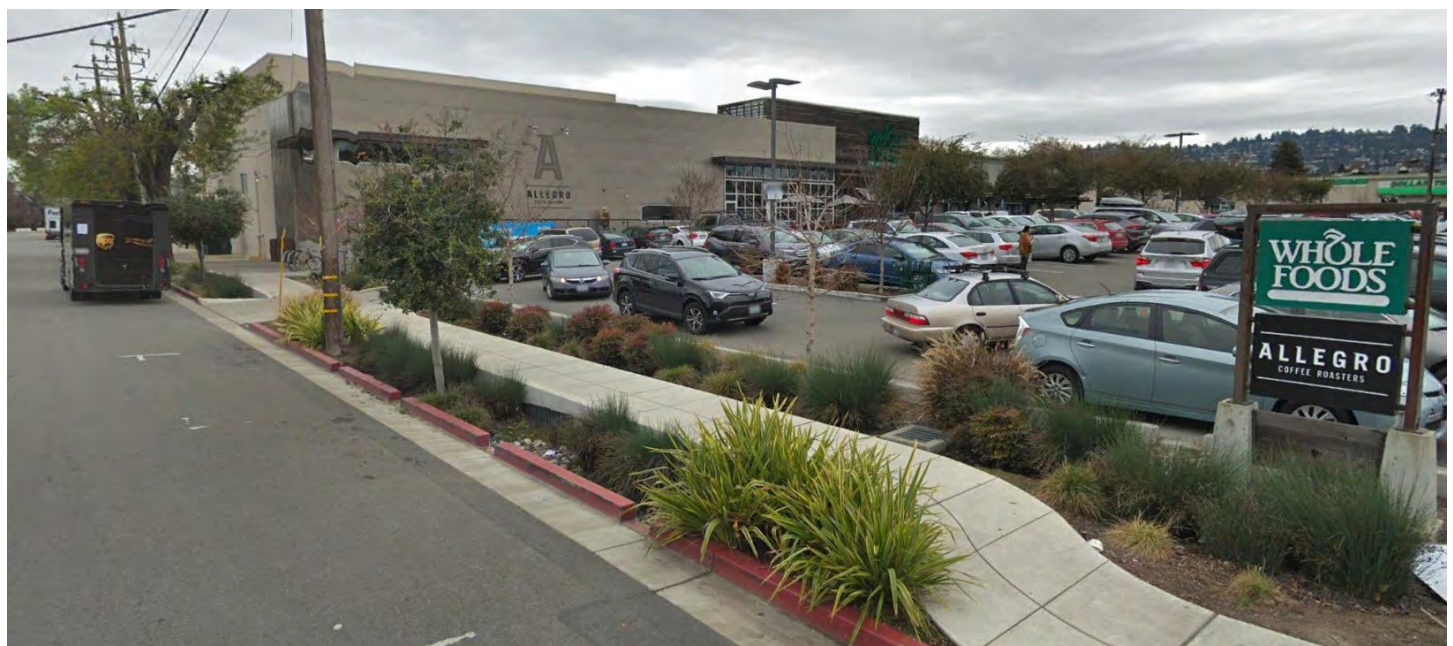
FIGURE B-22: VEGETATED STORMWATER MANAGEMENT FACILITIES HELP CAPTURE AND TREAT STORMWATER AND INCREASE GREENERY IN DEVELOPED AREAS.PHOTO: GOOGLE EARTH
