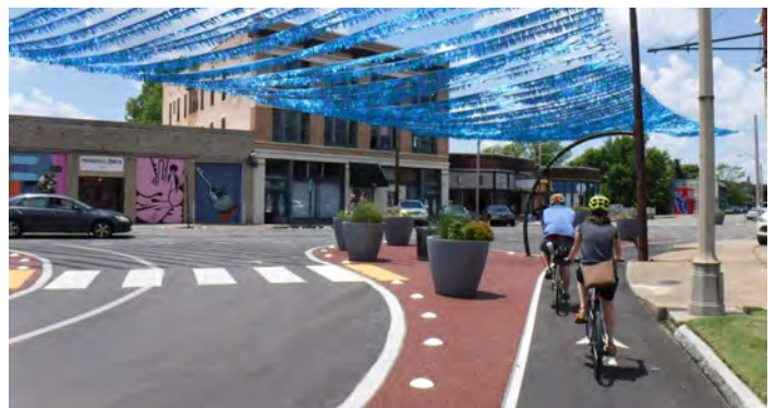
FIGURE B-23: CURB EXTENSIONS COMPRISED OF PLANTER BOXES IN MEMPHIS, TN. (PHOTO CREDIT: ALTA PLANNING + DESIGN)
